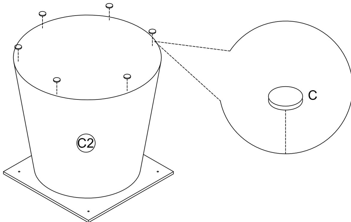
Step 2: Use Hex Key(D) to attach the Table Base(C2) to the Table Top(C1) with Bolt(A) and Washer(B).
